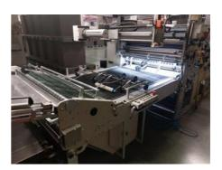
WPS 1100 - 2 window patching machine with a foil
